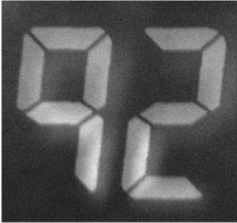
Figure 3. The displayed image using a dye-doped T-PDLC reflective display at V=20 V rms . White paper was placed behind the bottom substrate as a diffusive reflector. Black dye concentration: 2%, LC/polymer mixture: NOA65: E48=40:60, d=6.7 \mu m (11).
